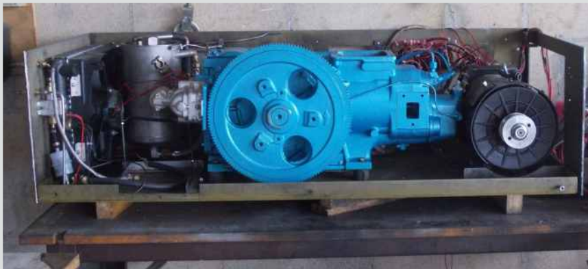
Auxiliary Power Unit (A.P.U.)
